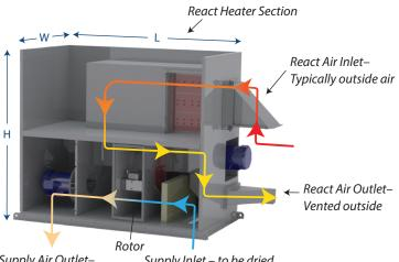
Supply Air Outlet– Supply Inlet – to be dried Dehumidified, dry air
